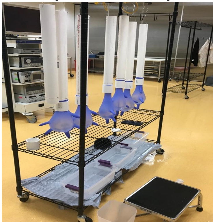
Figure note: Set up to test physical integrity of gloves using the water-leak method
